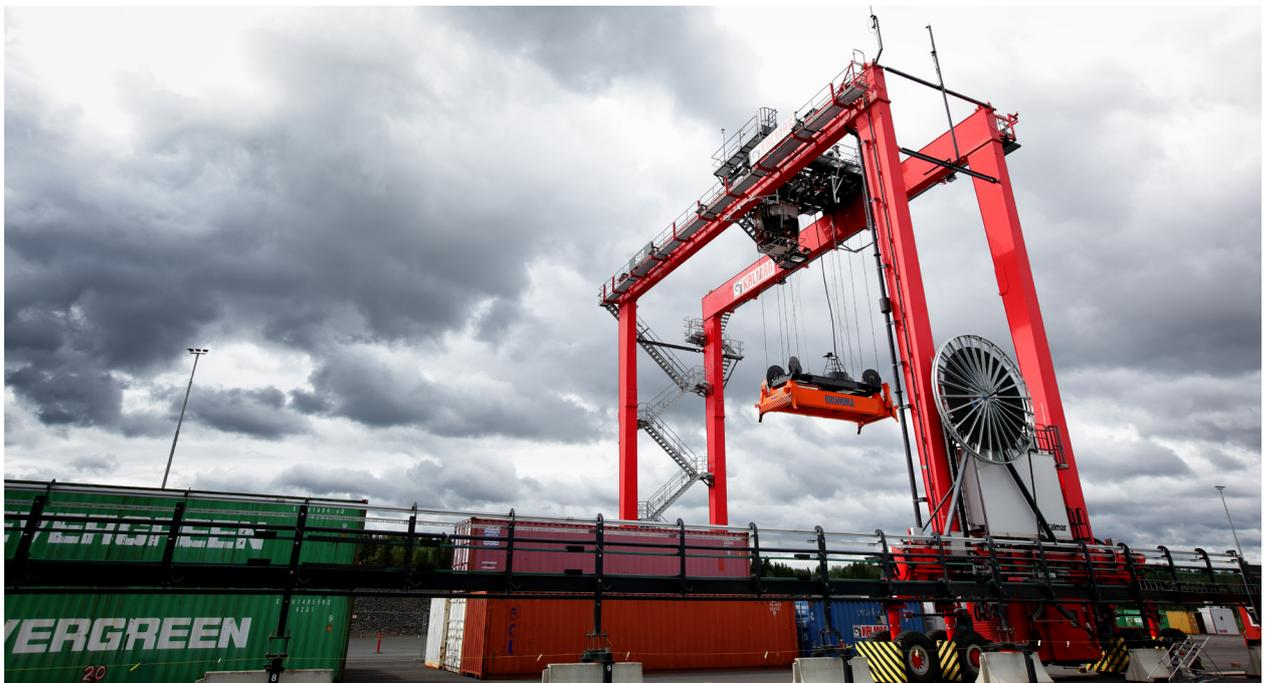
For RTG operations, a key safety consideration is container handling, both in the stack and during loading/unloading. Essential safety features in the truck lane include two-way audio capability that enables the truck driver to communicate with the remote operator in exceptional situations. For the operator, clear visibility to the truck lane via multiple camera views is crucially important.
