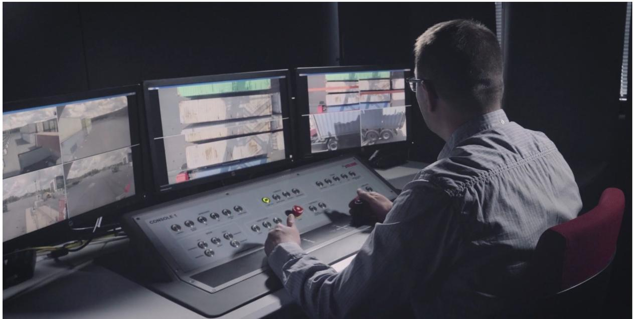
*The most significant cost savings from automation are due to the drastically smaller number of operators required. Typically, a single operator can handle two to three AutoRTGs remotely, and in quiet periods even up to six machines.*
